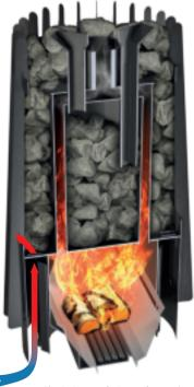
Ash falls through the plates of the grate into the ash drawer, which allows convenient cleaning of the heater without interruption of burning
