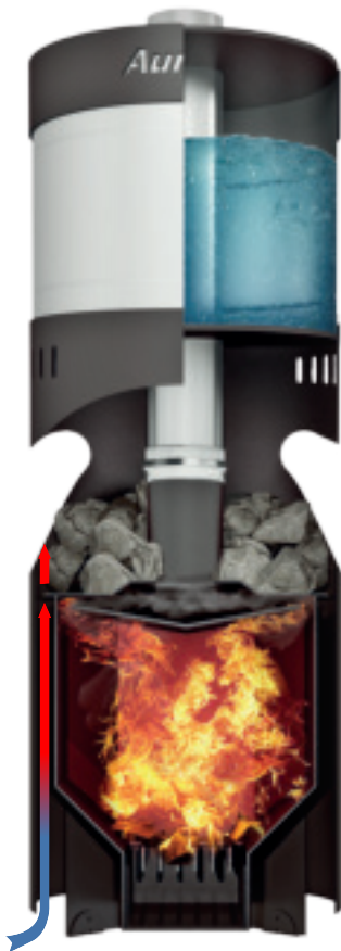
Fig. 4 Heater design and operation
