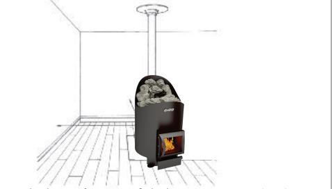
The clearance for an uncertified radiant stove is 1200 mm (48 in.) and for a stove with a sheet metal jacket or casing the clearance is 900 mm (36 in.). The clearances are large because they apply to all shapes, sizes and designs of stoves that have not been tested to determine the actual clearances.
