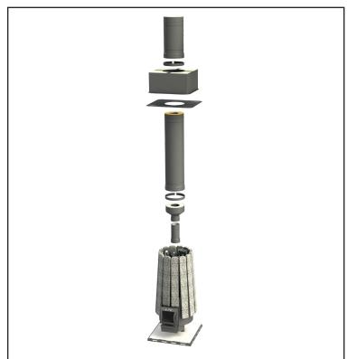
The ideal single-wall flue pipe assembly runs straight up from the stove. Straight venting systems produce stronger draft and will need less maintenance than if the assembly has elbows. A straight single-wall flue pipe assembly needs an inspection sleeve or telescopic section so it can be installed and removed without having to move the appliance. The sleeve also allows some movement for expansion when the flue pipe gets hot.
